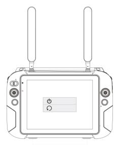
Figure 3-21 Turn the Remote Controller Off or Restart
