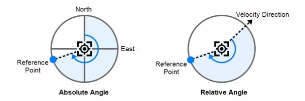
Figure 4-42 Absolute Angle and Relative Angle
