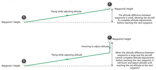
Figure 4-21 Waypoint Route Flight Altitude Transfer
