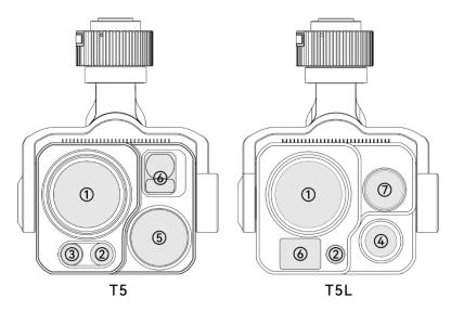
Figure 3-8 Gimbal Camera Adapted for Aircraft
