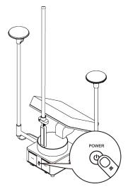
Figure 3-14 Turn on the tracking antenna
