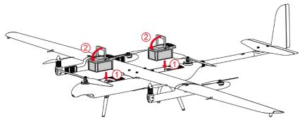
Figure 4-8 Assemble the battery
