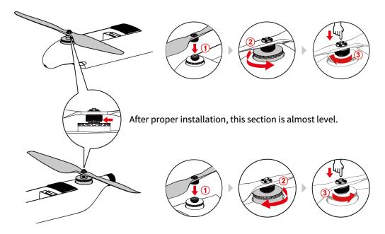
Figure 4-6 Assemble propeller
