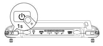
Figure 3-20 Turning the Remote Controller On
