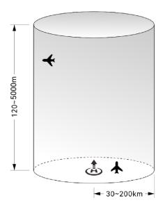
Figure 2-8 Diagram of Altitude and Distance Limits
