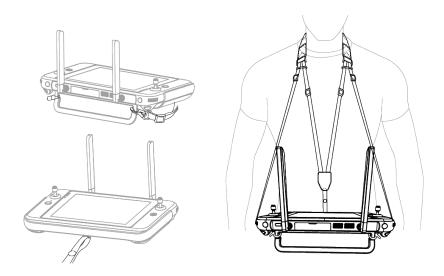
Figure 4-11 Install the Remote Controller Lanyard (As Required)
