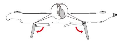
Figure 4-1 Open the landing gear
