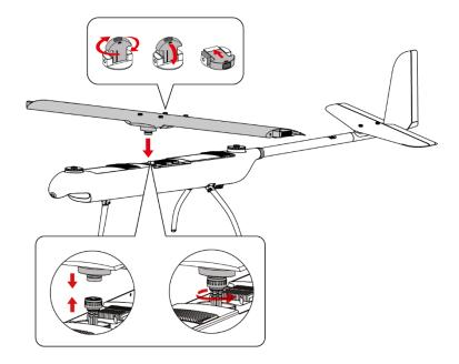
Figure 4-3 Assemble the central wing
