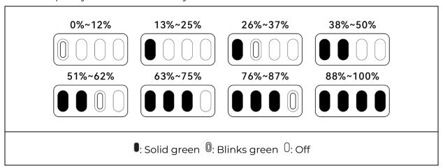
Figure 3-5 Battery Level Indicator Status (Non-Charging Status)
