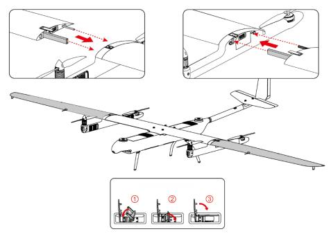
Figure 4-5 Assemble the left wing and right wing
