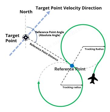
Figure 4-45 Figure-8 Circling Tracking
