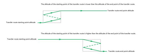
Figure 4-49 Transfer Route Altitude Adjustment
