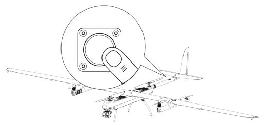
Figure 4-9 Turning the Aircraft On
