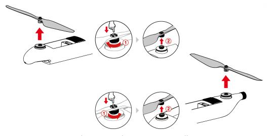
Figure 4-7 Disassemble propeller
