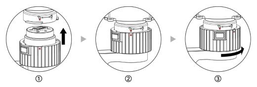
Figure 3-9 Install a Gimbal Camera on the Aircraft
