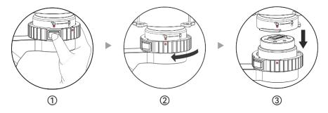
Figure 3-10 Uninstall the Gimbal Camera from the Aircraft
