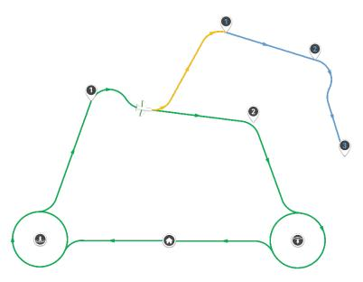
Figure 4-48 Perform Temporary Missions by Diverting Routes (Orange)
