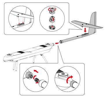
Figure 4-2 Assemble the tail wing
