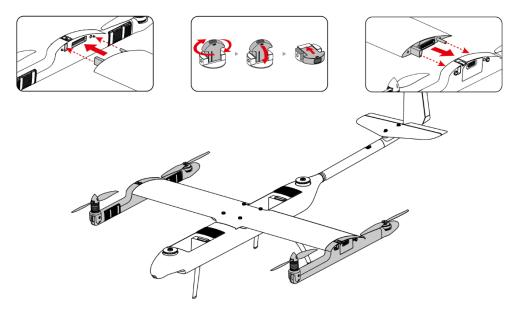
Figure 4-4 Assemble the left nacelle and right nacelle
