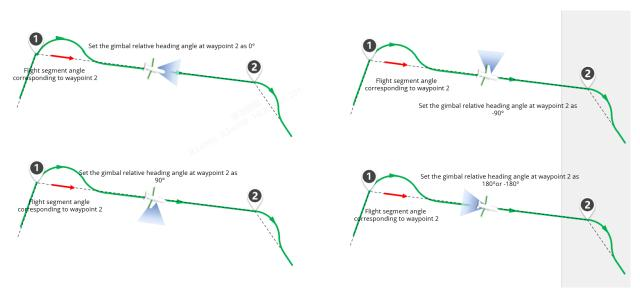
Figure 4-25 Description of Gimbal Relative Heading Angle
