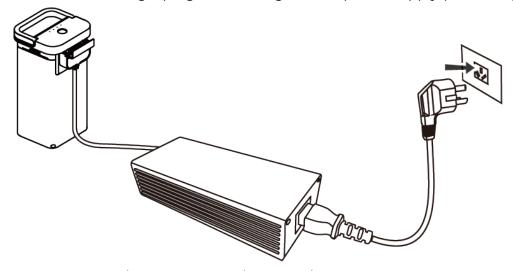
Figure 3-16 Charging Tracking Antenna
