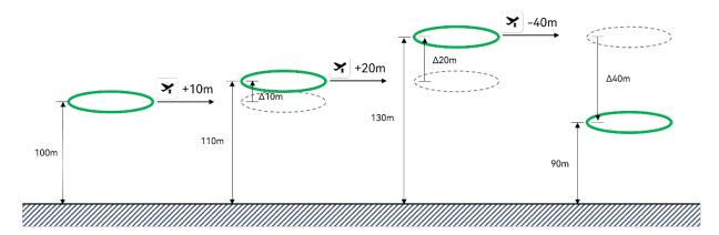
Figure 4-54 Change Altitude Logic Multiple Times with One Click
