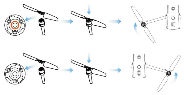
Fig 3-5 Install the Propellers
