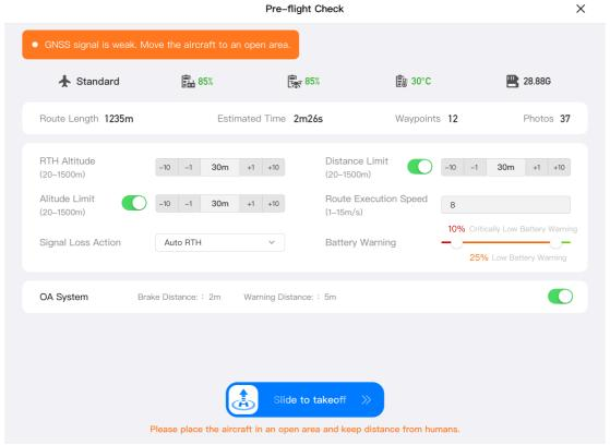
Fig 6-26 Pre-flight Check for a Flight Mission
