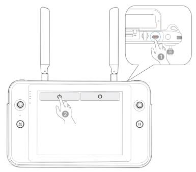
Fig 4-7 Turning the Remote Controller Off
