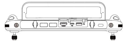
Fig 4-16 Custom Keys C1 and C2
