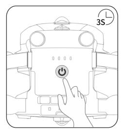
Fig 5-2 Turn On or Off the Smart Battery
