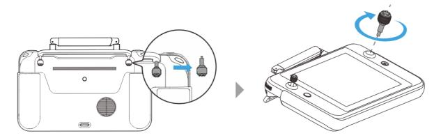
Fig 4-5 Installing command sticks
