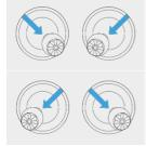
When the aircraft is in landing state, simultaneously move the left and right sticks inward or outward, as shown in the figure, until the motor stops.
