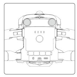
Fig 2-1 Front and rear visual lens modules of the aircraft
