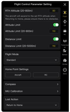
Fig 6-6 "Flight Control Parameter Setting" interface
