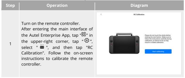
Calibration of the dials command sticks: According to the calibration guide page of the remote controller, move the left and right dial wheels and the left and right sticks according to the directions shown in the figure and hold for 1 second. At this time, a beep will be heard, and the calibration direction icon will be changed from gray to dark blue, indicating that the orientation calibration was successful.
