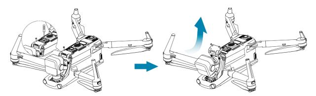
Fig 3-13 Removing the Gimbal
