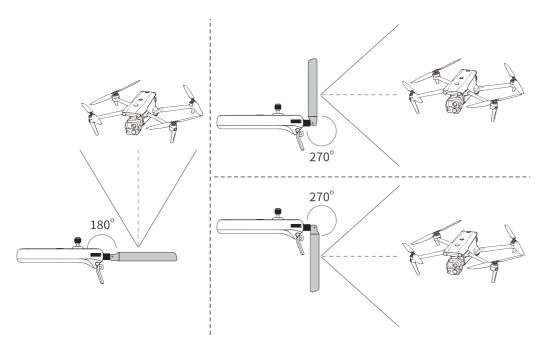
Fig 4-10 Extend the antenna
