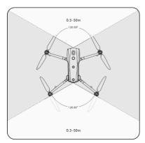
Fig 2-3 Observation Range of Millimeter-wave Radars
