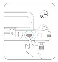
Fig 4-6 Turning the Remote Controller On
