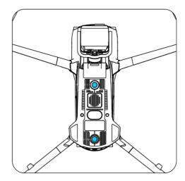
Fig 2-2 Top and bottom visual lens modules of the aircraft
