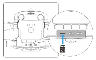
Fig 3-15 Installing the microSD Card
