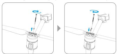
Fig 3-7 Install the Propellers
