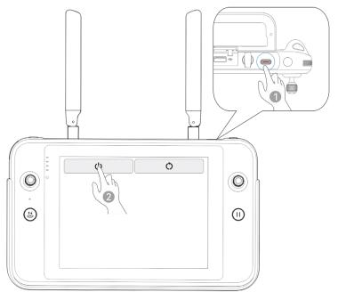
Fig 4-7 Turning the Remote Controller Off
