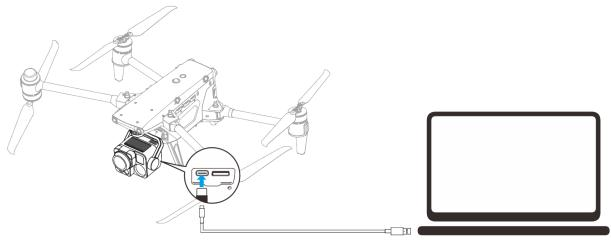
Fig 3-18 Connect to PC/MAC via Gimbal USB-C Interface
