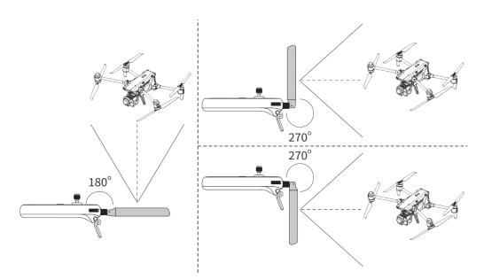
Fig 4-10 Extend the antenna
