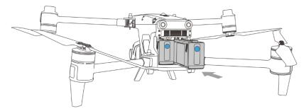
Fig 5-2 Install the Smart Battery
