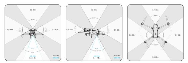
Fig 2-3 Observation Range of Millimeter-wave Radars
