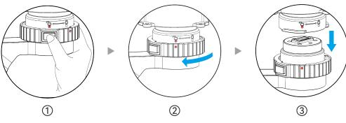
Fig 3-16 Removing the Gimbal
