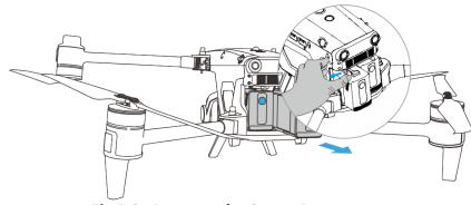
Fig 5-3 Remove the Smart Battery
