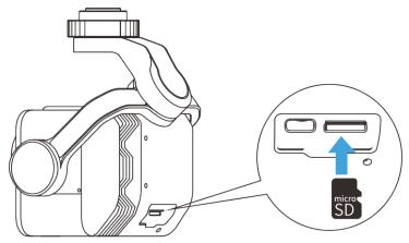
Fig 3-17 Installing the microSD Card
