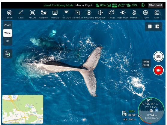
Fig 6-17 "Wide Angle Camera" Interface
