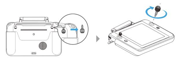
Fig 4-5 Installing command sticks
