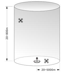
Fig 2-4 Diagram of altitude and distance limits
