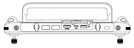
Fig 4-16 Custom Keys C1 and C2
