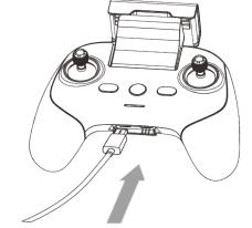
Fig 4-3 Use the Charger to Charge the RC
