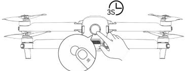
Fig 5-2 Turn On or Off the Smart Battery
