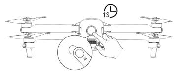
Fig 5-3 Checking Battery Level
