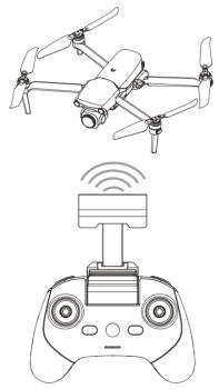
Fig 4-6 Extend the Antenna
