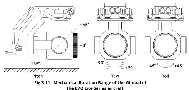
The mechanical rotation ranges of the pitch, yaw, and roll axes of the gimbal are shown below.
