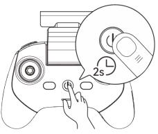
Fig 4-5 Turn the RC On
