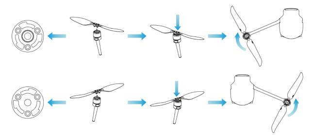
Fig 3-5 Install the Propellers
