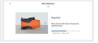
Place the nose of the aircraft flat on the ground until the next step is displayed. Be careful not to knock the front visual sensor.
