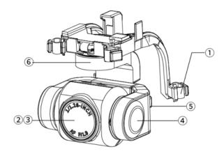
Fig 3-8 Gimbal Structure of EVO Nano+ Aircraft
