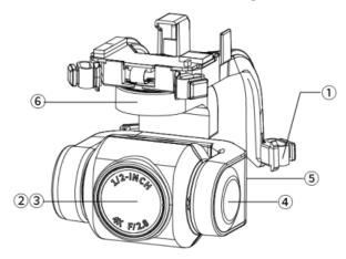
Fig 3-7 Gimbal Structure of EVO Nano Aircraft
