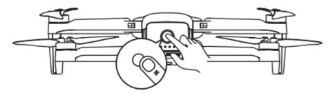
Fig 5-3 Checking Battery Level
