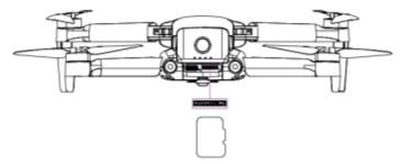
Fig 3-10 install a microSD Card
