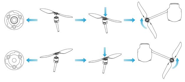
Fig 3-5 Install the Propellers
