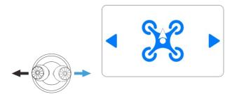
The left-and-right direction of the right stick is the roll stick, which is used to control the flight of the aircraft in the left and right directions.
