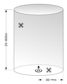
Fig 2-2 Altitude and Distance Limitation Diagram
