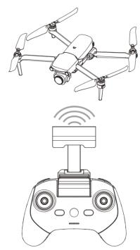
Fig 4-6 Extend the Antenna
