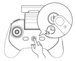
Fig 4-5 Turn the RC On
