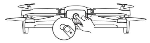
Fig 5-2 Turn On or Off the Smart Battery
