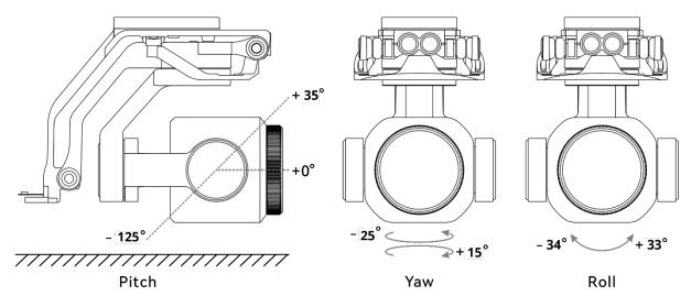
Fig 3-9 Mechanical Rotation Range of the Gimbal of the EVO Nano Series aircraft
