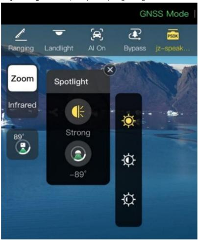
2. Adjust angle: adjust the spotlight irradiation (gimbal) angle.
