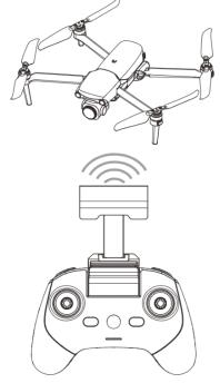
Fig 4-6 Extend the Antenna
