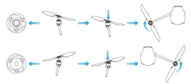
Fig 3-5 Install the Propellers
