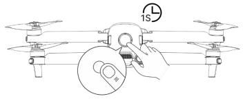
Fig 5-3 Checking Battery Level
