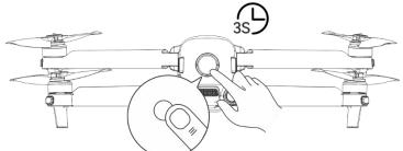
Fig 5-2 Turn On or Off the Smart Battery
