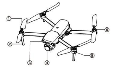
Fig 3-1 Aircraft Overhead View
