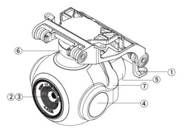
Fig 3-9 Gimbal Structure of EVO Lite Aircraft
