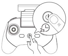
Fig 4-5 Turn the RC On
