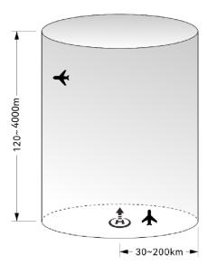
Fig 2-7 Diagram of altitude and distance limits
