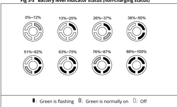
Fig 3-5 Battery level indicator status (non-charging status)
