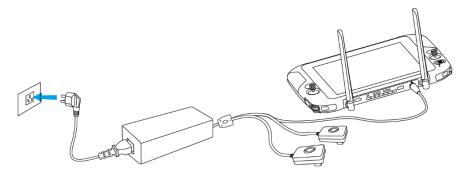
Fig 3-22 Use the charger to charge the remote controller
