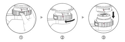
Fig 3-12 Remove the gimbal camera from the aircraft
