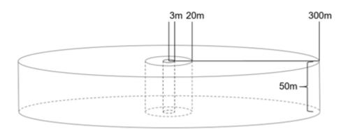
Fig 4-56 Return Area Diagram (Cylinder with the lower surface at the switching altitude)
