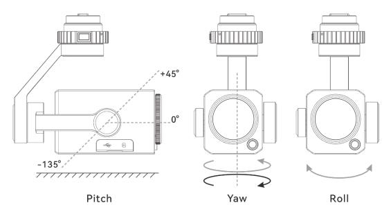
Fig 3-10 Description of the mechanical rotation range of the gimbal (the picture above shows the Z2)
