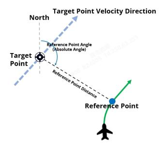
Fig 4-40 Synchronous tracking
