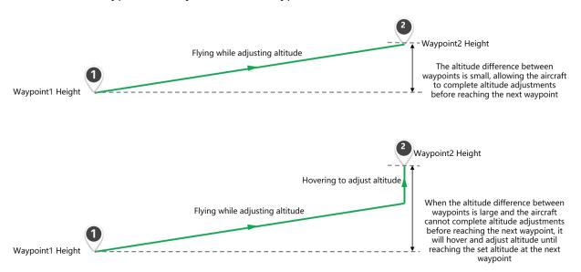
Fig 4-19 Waypoint route flight altitude transfer
