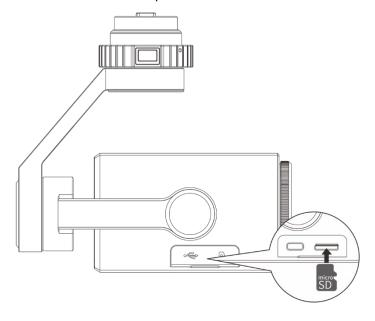
Fig 3-13 Install a TF card on gimbal camera
