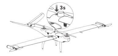
Fig 4-4 Aircraft powering on
