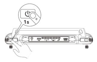
Fig 3-20 Turning the Remote Controller On
