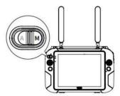
Fig 4-29 When the RC mode is M mode
