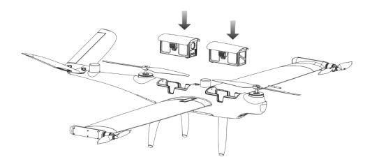
Fig 4-3 Install the Smart Battery
