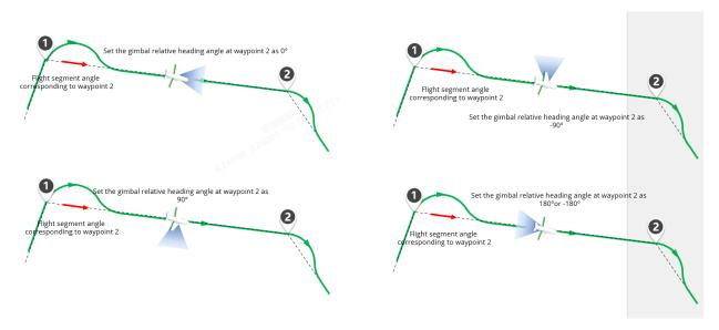
Fig 4-23 Description of gimbal relative heading angle
