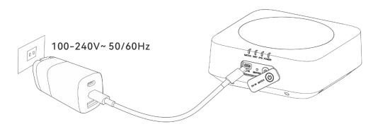
Fig 3-16 Charge the base station via base station charger
