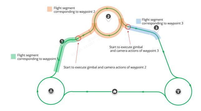
Fig 4-21 The flight segment corresponding to the waypoint
