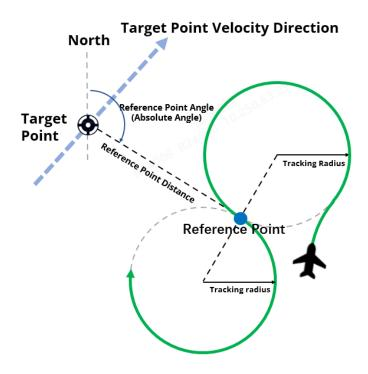
Fig 4-39 Figure-8 circling tracking
