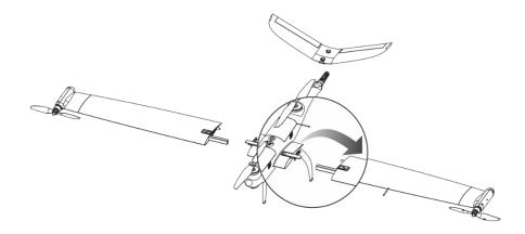
Fig 4-1 Install the wings
