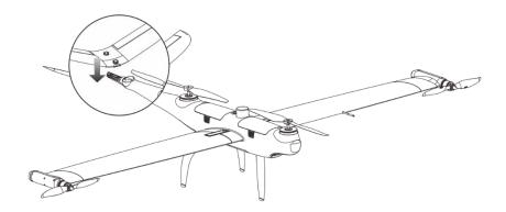
Fig 4-2 Install the rear wing
