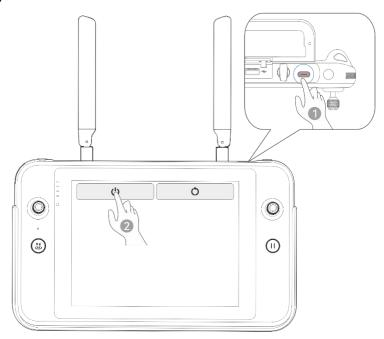
Fig 4-7 Turning the Remote Controller Off
