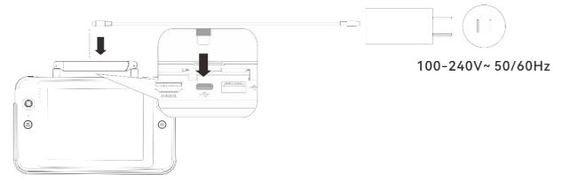
Fig 4-9 Use the RC charger to charge the remote controller
