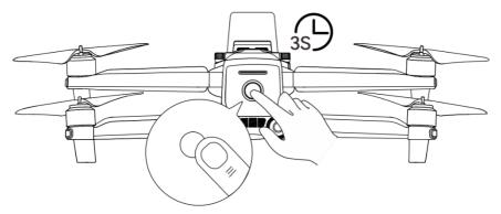
Fig 5-2 Turn On or Off the Smart Battery
