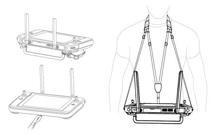
Fig 4-4 Install the Remote Controller Lanyard (As Required)
