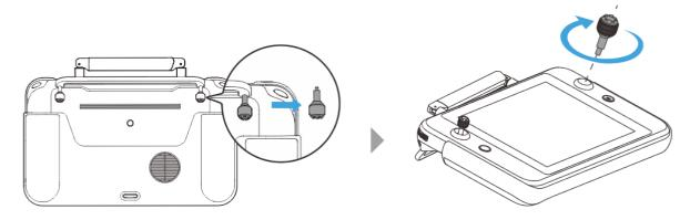
Fig 4-5 Installing command sticks
