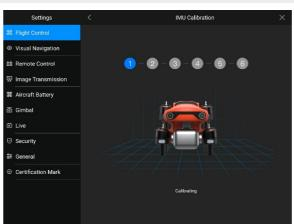
Flip the aircraft 180°, placing it with the belly facing up on a flat surface, until the App prompts you to proceed to the next step. Please be careful to protect the lens on the back of the aircraft during this process.
