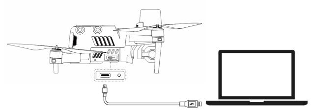
Fig 3-16 Connect the aircraft to PC/MAC
