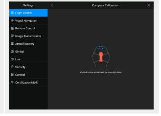
Hold onto the aircraft, positioning the nose to the left and the side facing downward.
