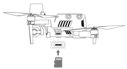
Fig 3-15 install microSD card
