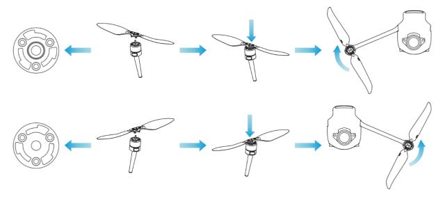
Fig 3-7 Install the Propellers
