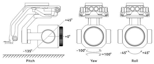
Table 3-11 Mechanical Rotation Range of the Gimbal of the EVO II RTK Series V3 Multi-rotor Drone
