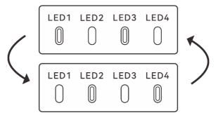
Fig 5-4 Self-heating State
