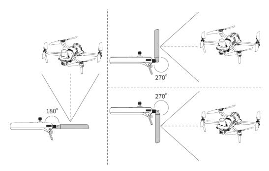
Fig 4-10 Extend the antenna
