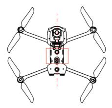
Fig 2-1 Recommended mounted area (bottom view)
