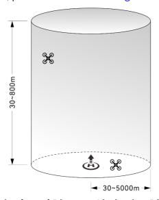
Fig 2-4 Altitude and Distance Limitation Diagram
