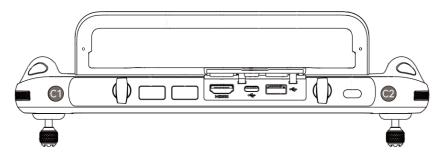
Fig 4-16 Custom Keys C1 and C2
