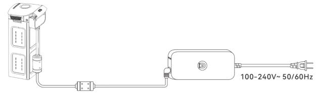
Fig 5-6 Use the Battery Charger to Charge the Smart Battery
