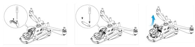
Fig 3-13 Removing the Gimbal
