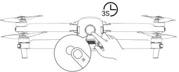
Fig 5-2 Turn On or Off the Smart Battery
