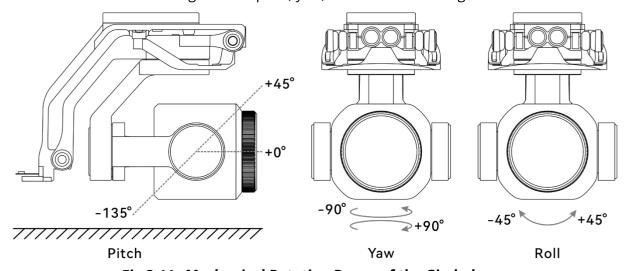
Fig 3-11 Mechanical Rotation Range of the Gimbal
