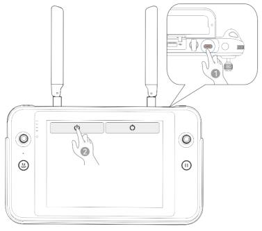
Fig 4-7 Turning the Remote Controller Off
