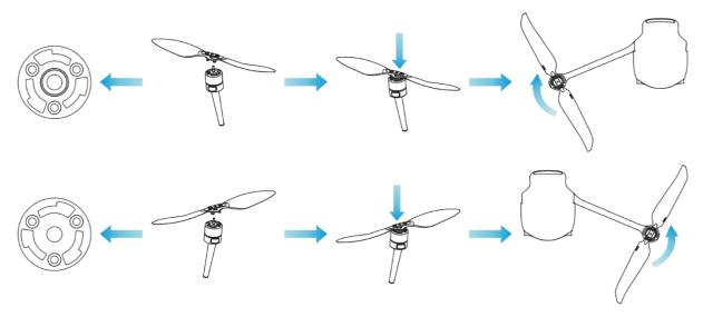
Fig 3-5 Install the Propellers
