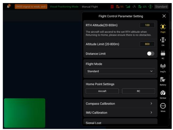
Fig 6-4 "Flight Control Parameter Setting" interface
