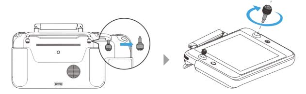
Fig 4-5 Installing sticks
