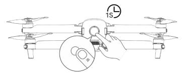
Fig 5-3 Checking Battery Level
