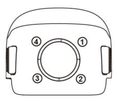
Fig 5-4 Distribution of Battery Level Indicator
