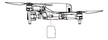
Fig 3-12 install a microSD Card
