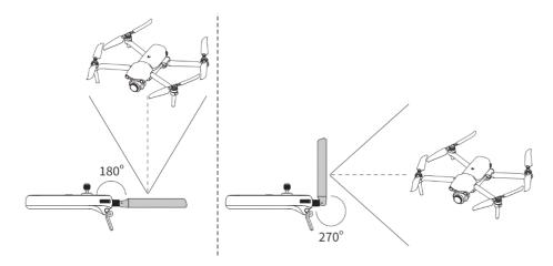
Fig 4-10 Extend the antenna
