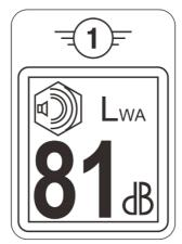
Fig 3-13 A-Weighted Sound Power Level of EVO Lite Enterprise Series multi-rotor drone
