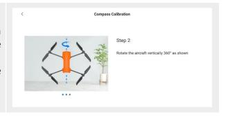
Hold onto the aircraft, positioning the nose to the left and the side facing downward.
