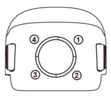
Fig 5-4 Distribution of Battery Level Indicator
