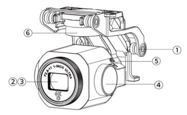
Fig 3-10 Gimbal Structure of EVO Lite+ Aircraft
