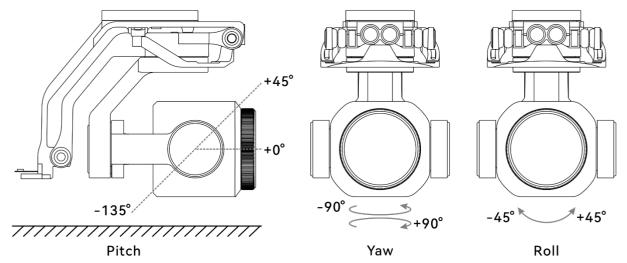
Fig 3-11 Mechanical Rotation Range of the Gimbal of the EVO Lite Series Multi-rotor Drone
