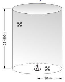
Fig 2-2 Altitude and Distance Limitation Diagram
