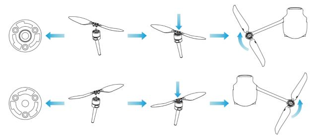
Fig 3-5 Install the Propellers
