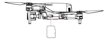
Fig 3-12 install a microSD Card
