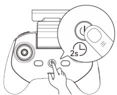
Fig 4-5 Turn the RC On
