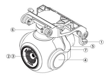
Fig 3-9 Gimbal Structure of EVO Lite Aircraft
