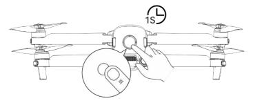
Fig 5-3 Checking Battery Level
