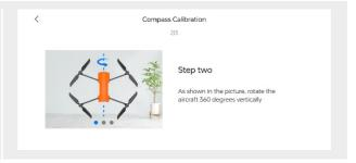
Hold onto the aircraft, positioning the nose to the left and the side facing downward.
