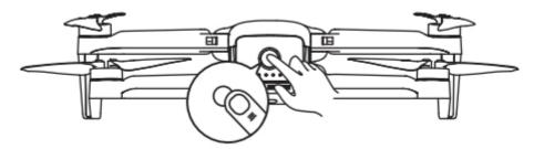
Fig 5-3 Checking Battery Level
