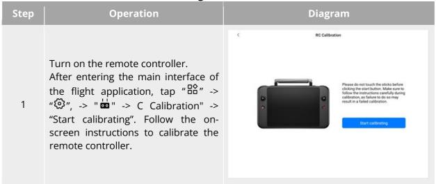
Calibration of the dials command sticks: According to the instructions on the calibration interface, move the left and right dial wheels and the left and right sticks according to the directions shown in the figure and hold for 1 second. At this time, a beep will be heard, and the calibration direction icon will be changed from gray to dark blue, indicating that the orientation calibration was successful.
