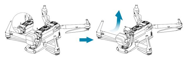
Fig 3-13 Removing the Gimbal
