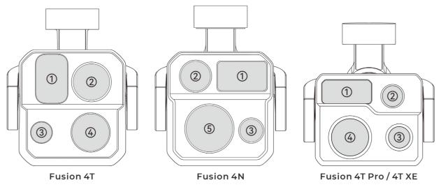
Fig 3-10 Aircraft Gimbal Camera Layout
