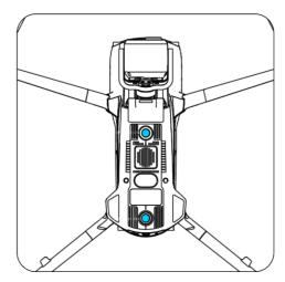
Fig 2-3 Top and bottom visual obstacle avoidance lens modules of the aircraft
