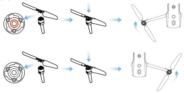
Fig 3-5 Install the Propellers
