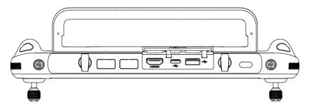
Fig 4-16 Custom Keys C1 and C2
