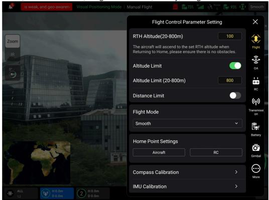
Fig 6-5 Setting Interface (Flight Control Parameter Setting)
