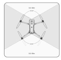
Fig 2-4 Observation Range of Millimeter-Wave Radars
