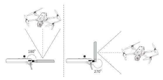
Fig 4-10 Extend the antenna
