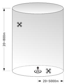
Fig 2-5 Diagram of altitude and distance limits
