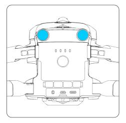
Fig 2-2 Front and rear visual obstacle avoidance lens modules of the aircraft
