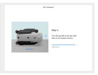
Fold the arms, turn the aircraft nose up, and lay it on the leveled surface 6 until interface the prompts calibration success. Be careful not to bump the rear camera lens.
