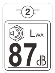
Fig 3-17 A-weighted sound power level of the drone
