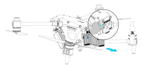
Fig 5-3 Remove the Smart Battery
