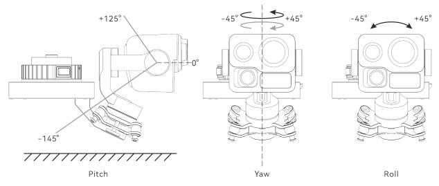
Fig 3-14 Mechanical Rotation Range of the Gimbal
