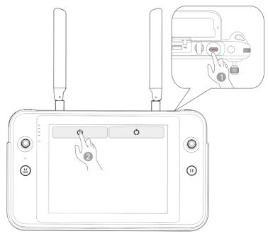
Fig 4-7 Turning the Remote Controller Off
