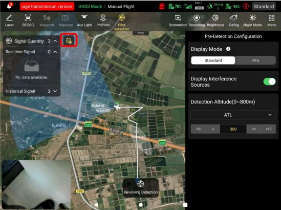
Fig 7-6 Pre-Detection Configuration.
