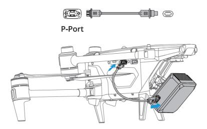
Fig 7-3 Data Cable Connection Diagram
