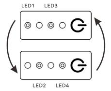
Fig 5-5 Self-heating State
