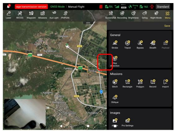
Fig 7-5 Adding Pilot Detection to the Main Function Bar.
