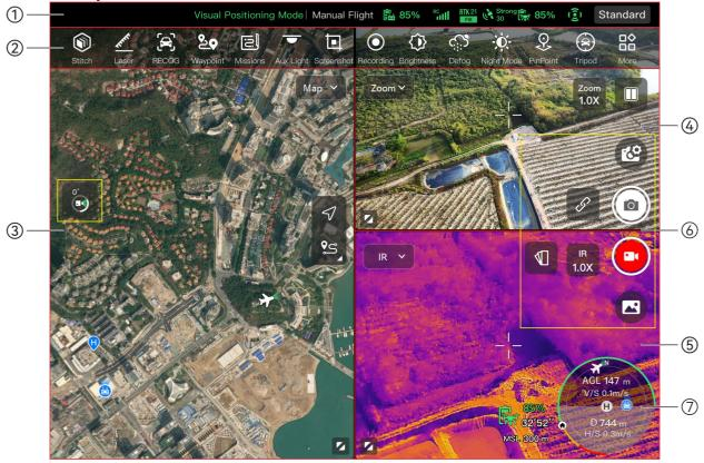
Fig 6-1 Main Interface of the flight application
