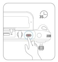
Fig 4-6 Turning the Remote Controller On
