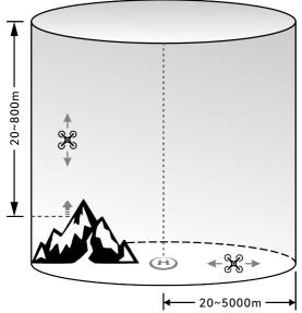
Fig 2-5 Diagram of altitude and distance limits
