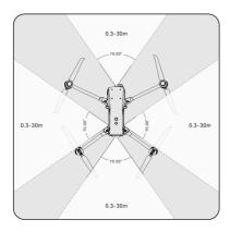
Fig 2-4 Observation Range of Millimeter-wave Radars
