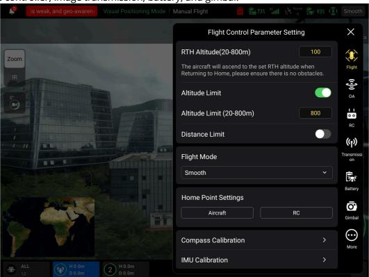
Fig 6-4 "Flight Control Parameter Setting" interface
