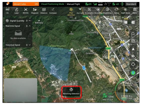
Fig 7-9 Automatic Rotational Detection Activation
