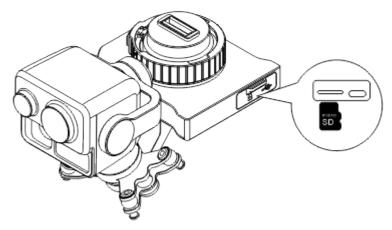
Fig 3-17 Installing the microSD Card
