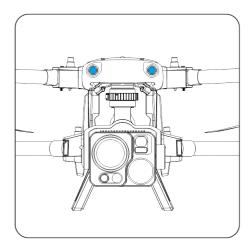
Fig 2-2 Front and rear visual lens modules of the aircraft
