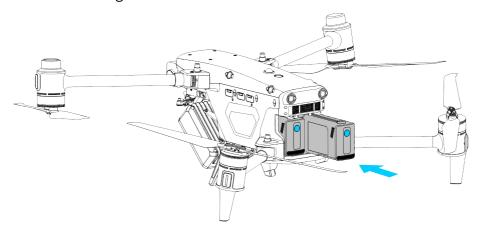
Fig 5-2 Install the Smart Battery
