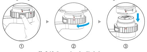
Fig 3-16 Removing the Gimbal
