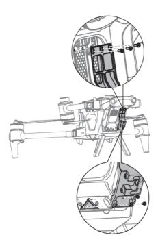
Fig 7-1 Adapter Bracket Installation Diagram
