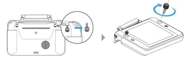
Fig 4-5 Installing command sticks
