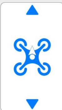
1. The up-and-down direction of the right stick is the pitch stick, which is used to control the flight of the aircraft in the forward and backward directions.
